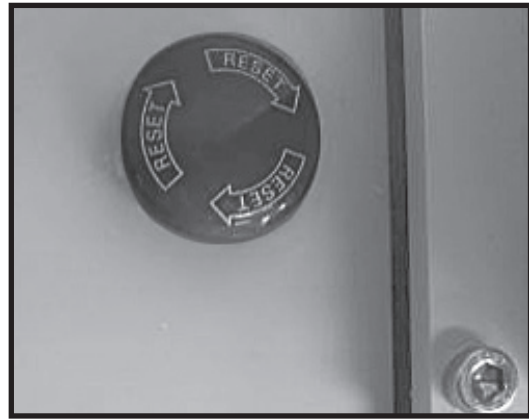
Emergency Stop button located on the side of the test next to the column. Turn the button Clockwise to release.
