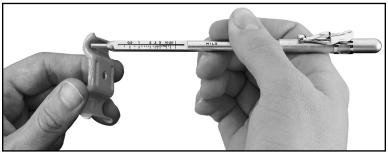
PosiPen has two scales, mils (inch) and microns (metric)
