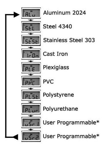
**NOTE:** If the Custom 1 and 2 are needed, they are set using the PC software (free) and downloaded to the gauge using the data cable (optional, p/n N-306-0010).
