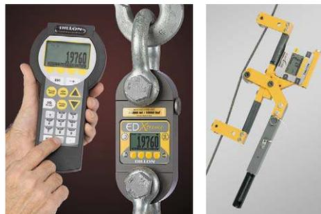
Dillon also manufactures electronic dynamometers and quick-attach tension meters.
