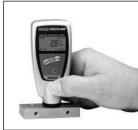
**NOTE:** After each measurement, lift the instrument a minimum of 0.12 in. (3 cm) from the measurement surface before you take another measurement.
