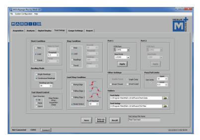
Configure test start and stop conditions.
