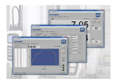
The programs include a set of tools to analyze test results, including statistical calculations, quick data export to Microsoft Excel, customizable reports, pass/fail indicators, and many others. Test setups are customizable and can be saved and recalled. The user can program test start and stop conditions, including load, time, distance, and sample break. Additional features include a large display screen for real time load and travel data and a utility to configure Mark-10 gauges from a PC.
