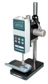
The ES05 is shown in a switch contact activation test, with Series BG digital force gauge, extension rod and rubber tip attachment.
