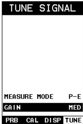
The screenshot shows a handheld device screen with a menu structure. At the top, 'TUNE SIGNAL' is displayed in a black bar. Below this, the screen is mostly blank. At the bottom, there are several menu items: 'MEASURE MODE P-E', 'GAIN MED' (which is highlighted with a black background), and 'PRB CAL DISP TUNE'.
