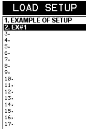
11) Use the **UP** and **DOWN** arrow keys to scroll through the setups until the target location to save the **Setup** is highlighted.
