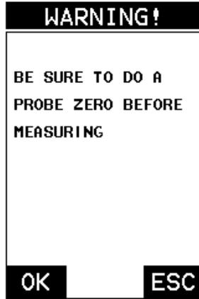
**Note:** When the zero probe option is set to manual, the probe zero disk (battery cap) located on the top of the gauge, will be used as a zero standard and the warning screen illustrated above will be displayed.
