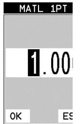
**NOTE: CHECK YOUR CALIBRATION!** Place the transducer back on the calibration point. The thickness reading should now match the known thickness. If the thickness is correct, repeat the steps above.
