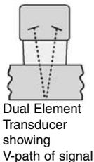
Dual element transducers are normally used in pulse-echo mode for finding defects, and in echo-echo mode for through coating measurements.
