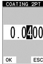
**NOTE:** CHECK YOUR CALIBRATION! Place the transducer back on both calibration points. The coating thickness readings should now match the known thickness values of each sample. If the thickness is not correct, repeat the steps above.
