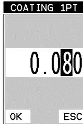
**NOTE: CHECK YOUR CALIBRATION!** Place the transducer back on the calibration point. The coating thickness reading should now match the known thickness. If the thickness is not correct, repeat the steps above.
