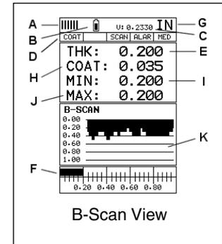
It's important to note that the measurement range on the display be set wide enough, so that the maximum thickness of the material can be viewed on the display. Using the diagram above, if the material thickness was actually 1.75", the underside of the material would not be viewable according to the current range at 0.00" – 1.00". All the user would see is a black screen from 0.00" – 1.00" with no view of the bottom contour at 1.75".
