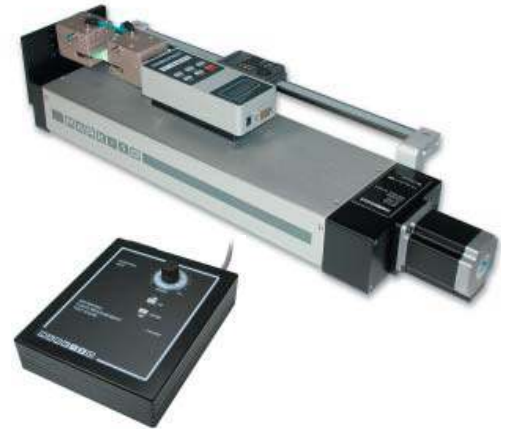
The ESMH is shown in a peel testing application, with Series BG digital force gauge, digital travel display, and pneumatic film & paper grips
