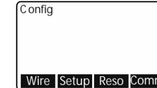
4. The unit is now in the Configuration mode. To see the rest of the softkeys available in this mode, press the **Right Arrow** key. All the Config softkeys are shown below.
