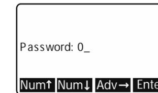
3. Use the **Num** and **Adv** keys to enter the Config password. Default is 0. After the number is displayed, press the **Enter** key. . .
