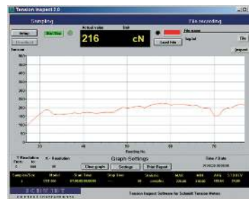
"Tension Inspect" software Main features: display of tension values, tension graph, storage of readings, statistics, set-up menu
