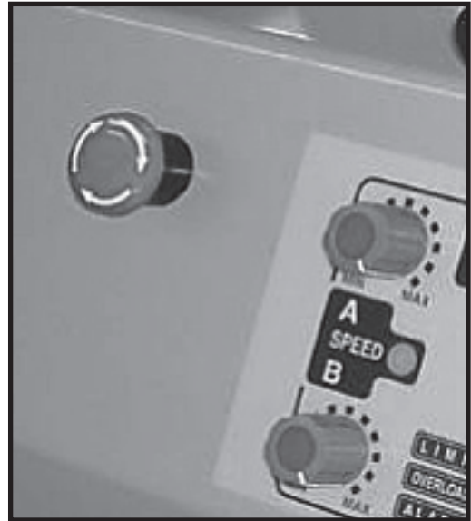
Emergency Stop button located on the side of the front plate. Turn the button Clockwise to release.
