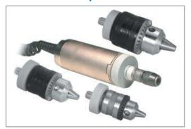
A great solution for general bi-directional torque testing applications with several different sample sizes. Three interchangeable chuck capacities and bit holder are available. The STH has superb overload protection and is available in capacities from 10 ozFin to 100 lbFin.
