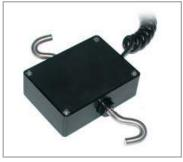
Measures tensile and compressive loads for a wide variety of applications, available in capacities from 0.25 lbF to 100 lbF. Threaded holes on two sides can accept a variety of hooks and implements, making this sensor particularly well suited for inline tests.
