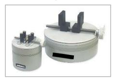
Ideal for testing torque on bottle caps and containers. Reversible jaws or movable posts, depending on model, effectively accommodate a variety of shapes and sizes. Capacities available from 10 ozFin to 100 lbFin.
