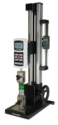
The ES30 is shown in a typical compression testing application, with Series 5 digital force gauge, digital travel display, and attachments
