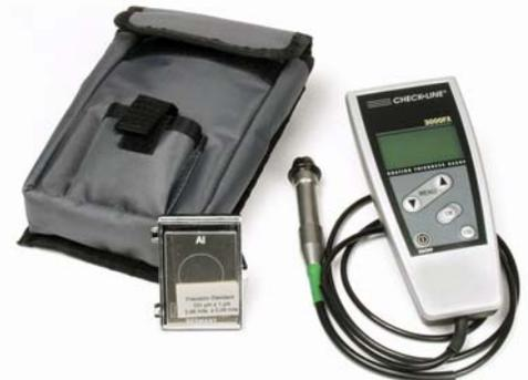
The 3000FX Series is supplied as a complete kit with gauge, ferrous and or non-ferrous zero plate (model dependent), 2 calibration standards, 2 AA batteries, carrying pouch, manual and manufacturer's calibration certificate.
