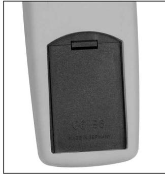
2. Open the battery compartment by pulling down on the tab located at the top of the battery cover and remove the cover. Insert two AA batteries following the orientation engraved on the inside of the battery compartment.
