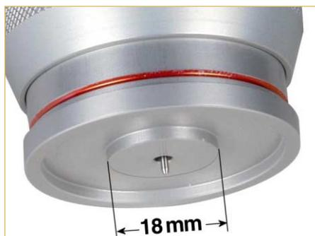
Oversized flat bottom design provides measurement stability for the "working face" (contact area) of the Durometer.
