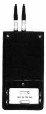
To exchange batteries you first have to unscrew the Phillips screw of the compartment cover. Then *carefully* lift the cover. Make sure that the rubber sealing of the cover will not be damaged or removed from the guiding notch. Insert new batteries. Ensure correct orientation according to the sketch. Reassembling is made in the reverse order.
