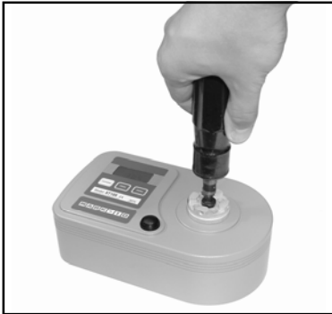
Fig. 1 Gradually exert torque to achieve accurate results
