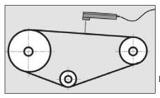
Figure 4. Measuring Free Belt Vibration Frequency
