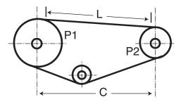
Figure 3. Measuring Free Belt Span (L)
