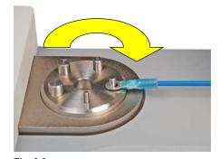
Fig. 3.1 Wire terminal fixture
