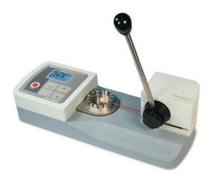
Thank you for purchasing a Mark-10 WT3-200 wire terminal pull tester, designed for pull test applications up to 200 lbF (1,000 N).
