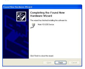
Click "Finish". The Mark-10 USB device is now installed and ready to use. The COM port number assigned by Windows may be identified in Device Manager, or in the communication application being used, such as MESURgauge or HyperTerminal.
