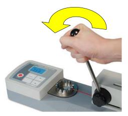
Fig. 3.4 Rotating the lever
